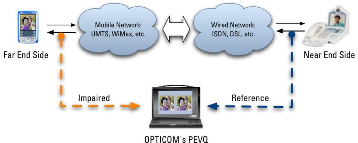
**Figure 5-1** A typical setup for an intrusive test: The tester outputs a reference stimulus that is inserted into a network connection at the 'near end side' (origin), while the received signal at the 'far end side' (termination) is fed back to the tester for difference analysis.
